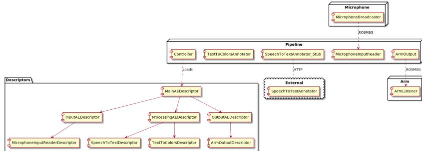
This diagram illustrates how the various components of our architecture connect together. Starting off in the bottom left corner is our **Descriptors** folder. This is a UIMA feature that allows the use of XML Descriptor files to define the structure of the data pipeline. This separation of structure from the functions of the code allows for less coupling between code units.
